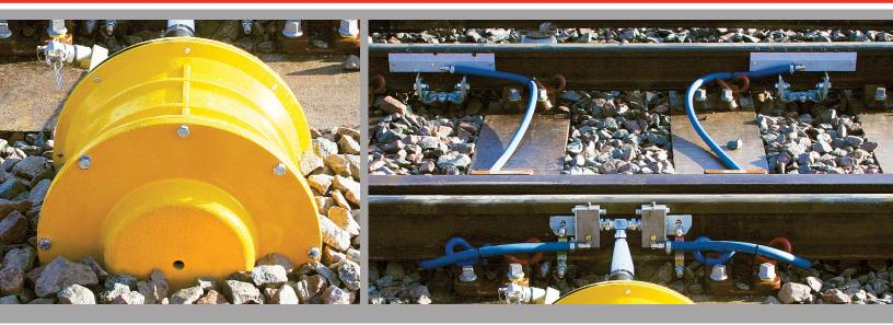
Distribution blades can be supplied in various lengths and the modular design enables easy installation and replacement with minimal blocking. There is simple blade height adjustment for precise delivery of grease to wheel flange and optional blade troughs to collect excess grease for easy cleaning. Blades can be fitted for high rail lubrication, check rail lubrication or both rails for reverse curve lubrication from one unit.
