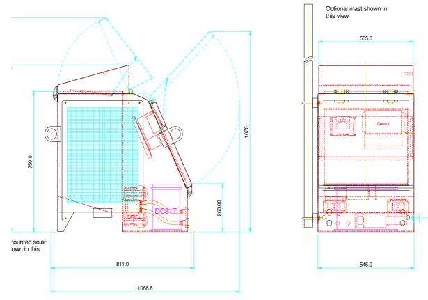
To install a LubriCurve Electro 15 lubricator, the cabinet has brackets with mounting holes for attaching directly to wooden sleepers or concrete base. The form and stability of the base is important as it resists the wind loads on the cabinet.
