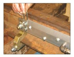
10.5.6 Set the blade to the required height below the railhead using a suitable gauge / measuring device. The minimum distance is 18mm. The precise height dimension is subject to rail profile and blade configuration and is covered in section 10.6. If required a suitable gauge is available from Whitmore Rail (Part No. LCS104-06), shows how to set the blade with the Whitmore Rail gauge).
