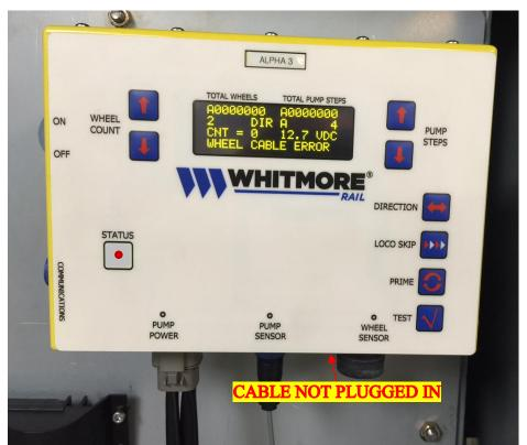
This error will only occur upon powering on the controller with the wheel sensor cable being unplugged or not having a good connection. The STATUS LIGHT (13) will illuminate red and the message WHEEL CABLE ERROR will display on line 4. To fix this power down the controller and ensure the wheel sensor cable is properly connected. You must power cycle the controller in order to clear the error. (<u>NOTE</u>: cables should never be connected/disconnected with the controller powered on)
