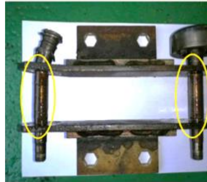
Wetted Pins observed during one of the maintenance activities –Good Oil Penetration
