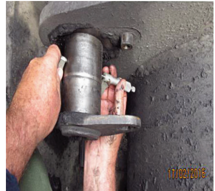
Bucket pin was measured at 3.536 inches (89.82mm).
