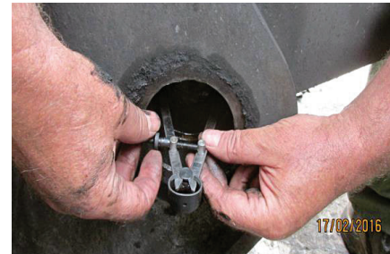
Bucket pin bushing was measured at 3.5555 inches (90.32mm).
